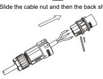
• Push the threaded sleeve into the socket, tighten up the cap on the terminal.
