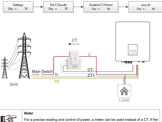
CT is fitted in the wrong orientation, anti-backflow function will fail.
