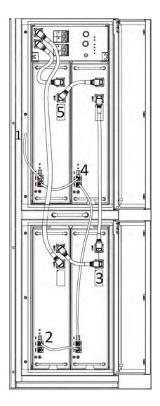
B. Connection of battery ground cable
