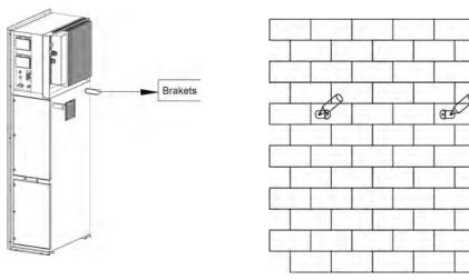
Drill holes on the marks with a diameter of 6mm drill. Insert the expansion screws into the hole.
