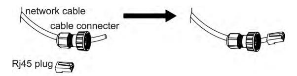
Step 4: Insert the cable connector into COM port at the bottom of energy station and screw it tightly. Then insert other side of the network cable into PC or other device.
