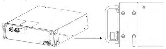
Push the battery into the All-In-One as shown in the figure below.
