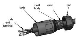
Install the cable into the plug terminal and lock the screw, torque is (0.8 + / - 0.1 N·m).
